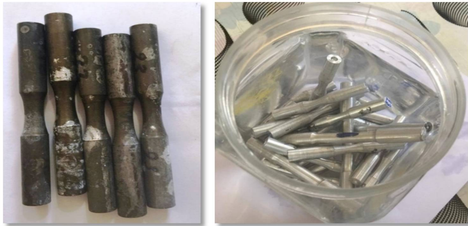
Figure 6: Container of 3.5% NaCl aqueous solution and samples after corroded by 3.5% NaCl
