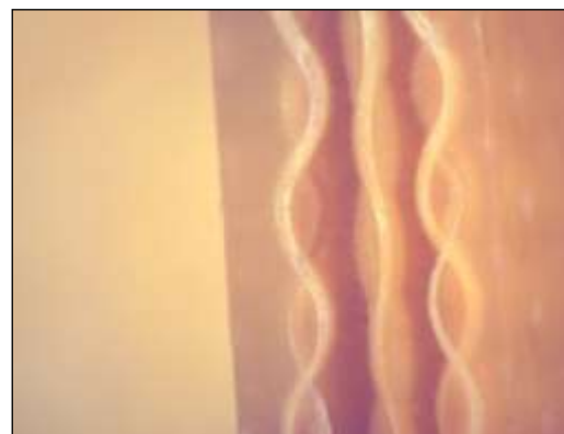
Figure (11) Optical micrographs of the prepared composite with three layers of the reinforcing material.
